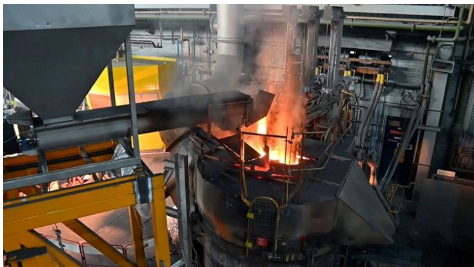
Figure 12: Addition of composite ore/reductant pellets to EAF during operation
